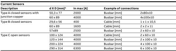
\*d: internal diameter - D: main external dimension
