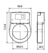
Current sensor type C Ø 100-120-200 mm up to 4000A Ø 290 mm from 2000A to 6300A
