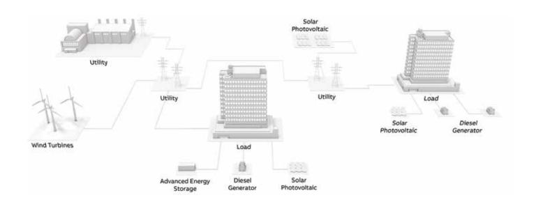
In order to maximize the service continuity, local generation starts to supply the islanded plant. Ekip UP integrates programmable status based on measurements, events and protections, so it is possible to create transfer switching logics. It can be also easily integrated with ATS controller in revamping projects.
